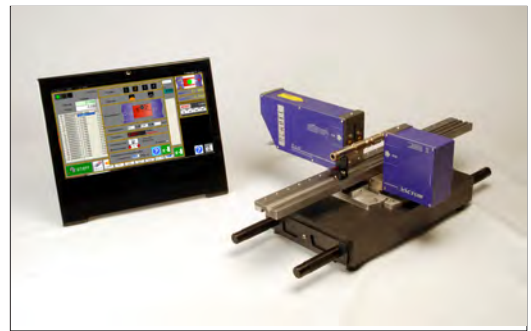
A Super Meclab 40 bench top laser micrometer
