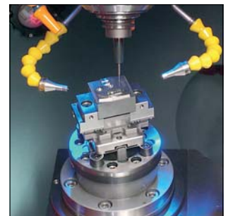
Ultra precision machining in hardened steel 47 HRC
